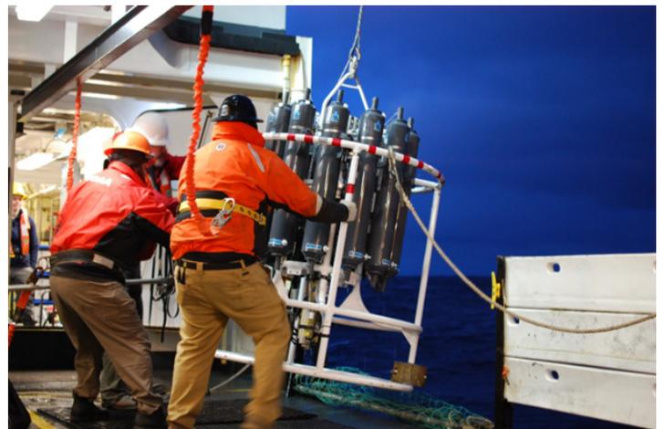
Conductivity, Temperature, and Depth sensor recovery on the NOAA *Bell M. Shimada*. Photo credit: Steve Lindley
